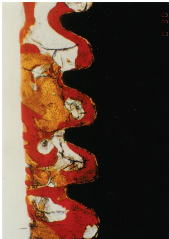
**Fig. 2.** HA coating appeared to have uniform thickness. Bone is in contact with implant surface along majority of implant surface (original magnification  $\times 4$ ). Gray lining along implant surface is HA coating, bone is stained red, and residual graft material is stained brown.
