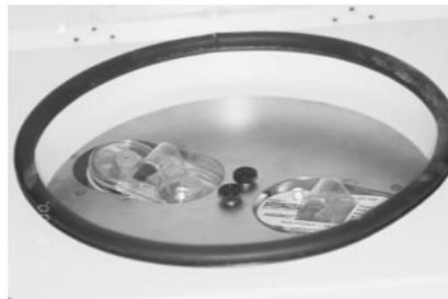
FIGURE 9. Chamber with blood placed into SmartPREP unit.
