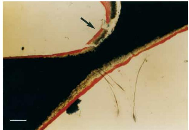
**Fig. 4.** Implant 13 years after loading: HA coating appears to form continuous layer along implant surface; bone appears in tight contact with coating and with detached HA coating fragments. *White line* represents 400  $\mu\text{m}$ . (Original magnification  $\times 4$ .)
