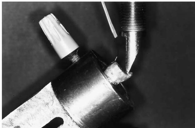
**Fig. 3.** External force was applied with universal testing machine at 45-degree angle to each crown.
