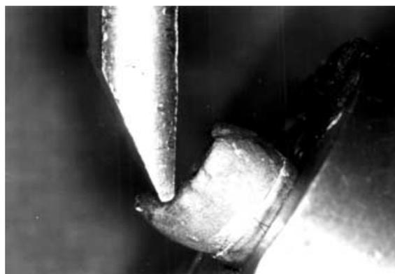
**Figure 3.** External force was applied at 45° angle through a Universal testing machine.
